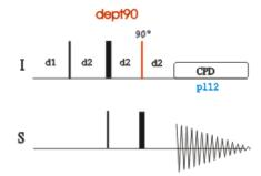
The time intervals depicted in the pulse sequence diagrams are not drawn to scale. For example, d1 is typically a few seconds while p1 is typically a few microseconds in length.
