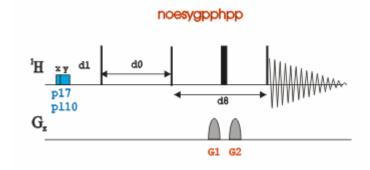
The time intervals depicted in the pulse sequence diagrams are not drawn to scale. For example, d1 is typically a few seconds while p1 is typically a few microseconds in length.
