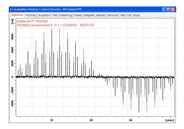
The POSMAX value of **p1** is displayed in the title window which is the 90° pulse, along with the experiment number and the NEXP value. Write this value down. To obtain a more accurate 90° pulse measurement, follow the steps below.
