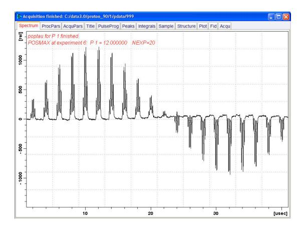
The POSMAX value of **p1** is displayed in the title window which is the 90° pulse, along with the experiment number and the NEXP value. Write this value down. To obtain a more accurate 90° pulse measurement, follow the steps below.
