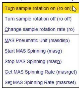
Rotation may be turned off for probes such as BBI, TXI, TBI and for small sample probes.
