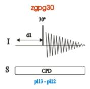
The time intervals depicted in the pulse sequence diagrams are not drawn to scale. For example, d1 is typically a few seconds while p1 is typically a few microseconds in length.
