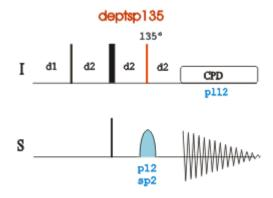
The time intervals depicted in the pulse sequence diagrams are not drawn to scale. For example, d1 is typically a few seconds while p1 is typically a few microseconds in length.
