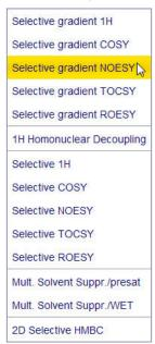
The default parameters are taken from the standard parameter set SELNOGP. The mixing time **D8** is dependent on the size of the Molecule and the magnetic strength. It can vary from a large Molecule to a small one from **100 ms** to **800 ms**.
