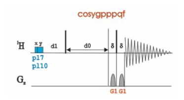
The time intervals depicted in the pulse sequence diagrams are not drawn to scale. For example, d1 is typically a few seconds while p1 is typically a few microseconds in length.
