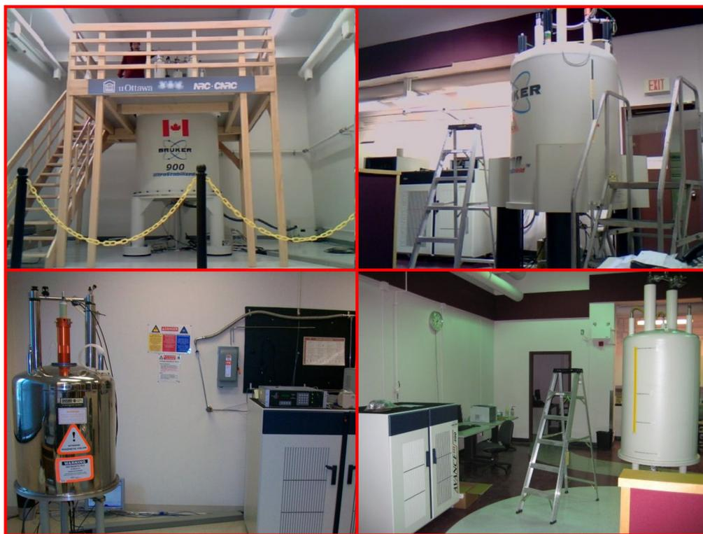
**Figure 1.2** Solid-state NMR spectrometers available at the University of Ottawa, as of 2011. Clockwise from upper left:  $B_0 = 21.1$  T;  $B_0 = 11.75$  T;  $B_0 = 9.4$  T;  $B_0 = 4.7$  T. All photos were taken by C. M. Widdifield during the period from April 2008 to August 2011.
