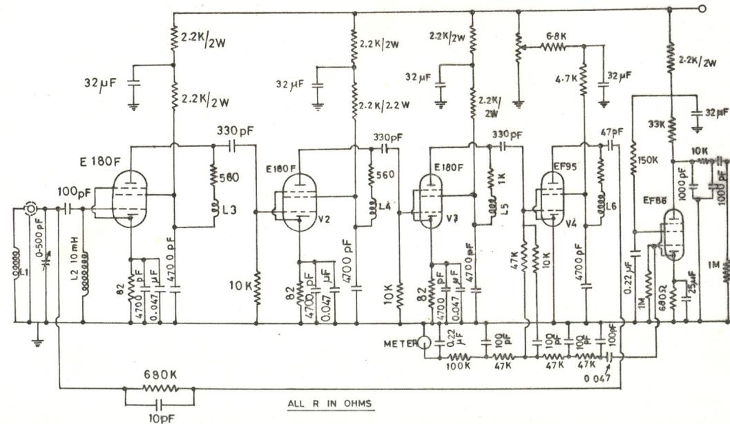
**Figure 2.2** Circuit diagram of Robinson oscillator.
