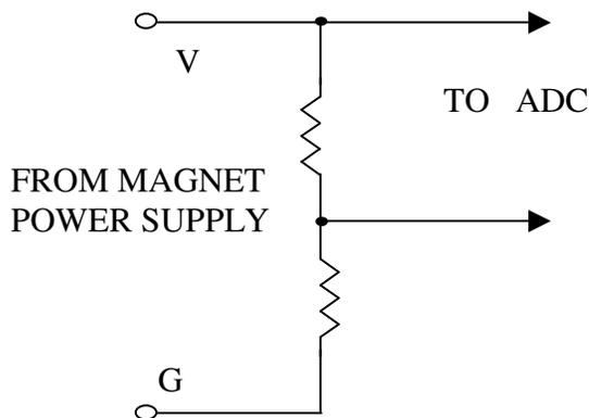
**Figure 2.9** Circuit diagram of the potential divider.
