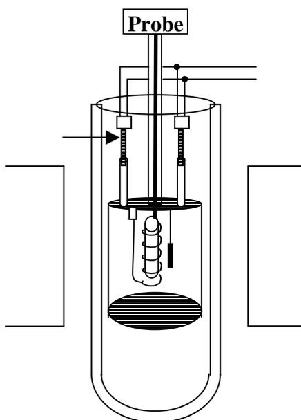
Figure 2.23 Variable temperature assembly (high temperature) (300 – 410 K).
