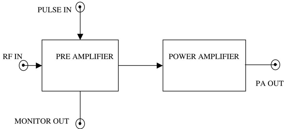
**Figure 2.17.** Block diagram of medium power amplifier.
