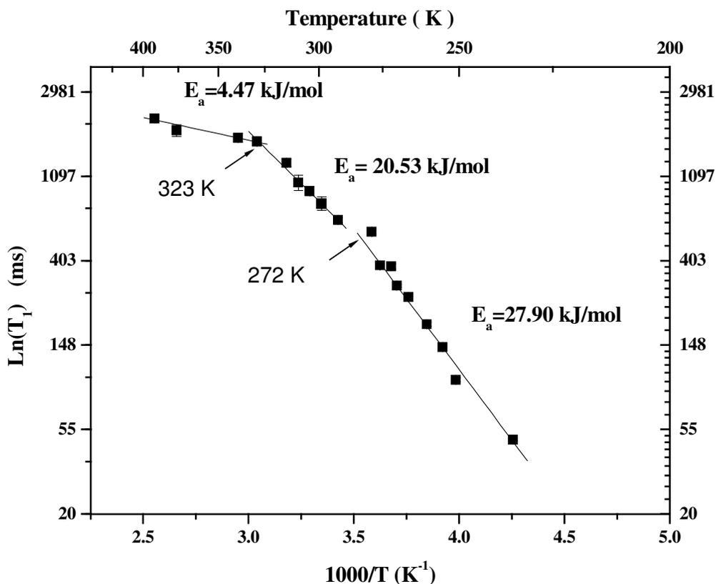
**Figure 5.2**  $T_1$  data in the temperature region 391-272 K. Solid lines represent straight line fit.
