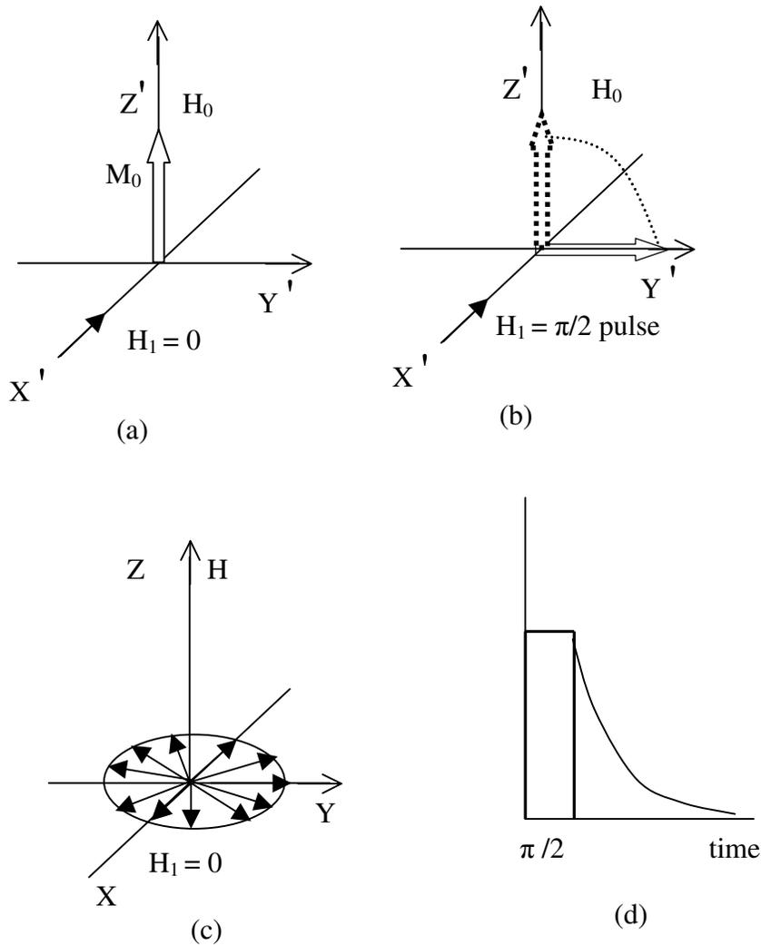
**Figure 1.6** (a) Equilibrium magnetization  $M_0$  when external rf field  $H_1 = 0$
