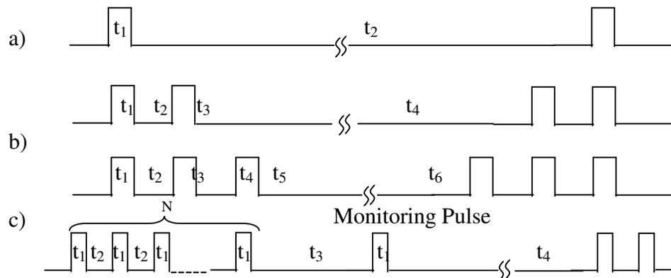
**Figure 2.14** Schematic representation of the different pulse sequences (a) Single pulse (b) Two pulse (c) Three pulse and (d) Saturation burst sequences.
