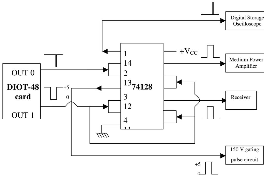
**Figure 2.15** Schematic representation of the buffer circuit.
