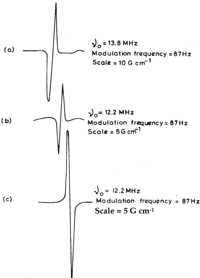
**Figure 2.5** <sup>1</sup>H NMR signal in glycerin with (a) field modulation and field sweep (b) frequency modulation and field sweep (c) field modulation and frequency sweep.
