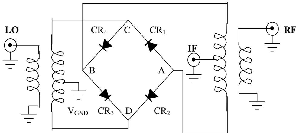
**Figure 2.18.** Schematic representation of a typical DBM.
