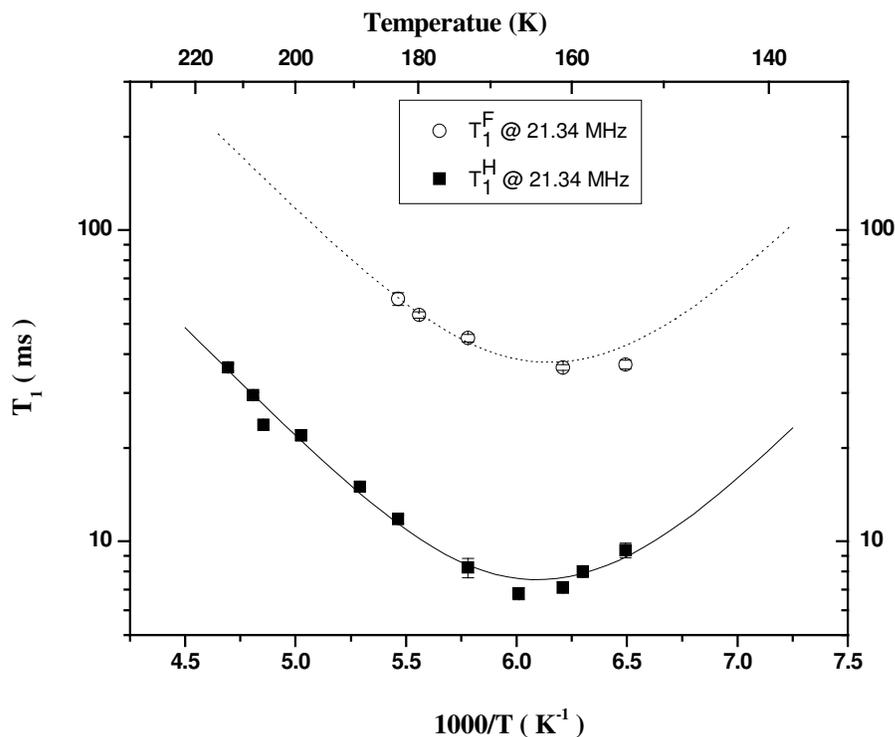
**Figure 3.5**  $^1\text{H}$  and  $^{19}\text{F}$   $T_1$  data in the temperature range 220 – 146 K. Solid line represents the BPP fit to  $^1\text{H}$   $T_1$  data and dotted line shows the simulated graph of BPP curve for  $^{19}\text{F}$   $T_1$  data.
