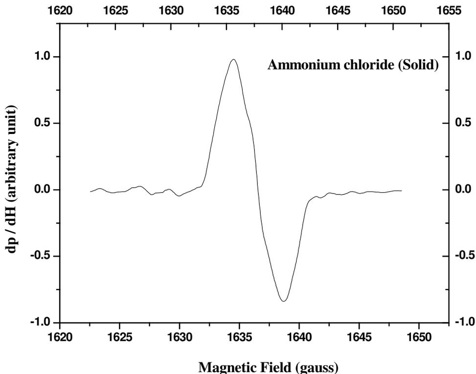
Figure 2.11. The  $^1\text{H}$  NMR signal in a solid  $\text{NH}_4\text{Cl}$  at 7 MHz.
