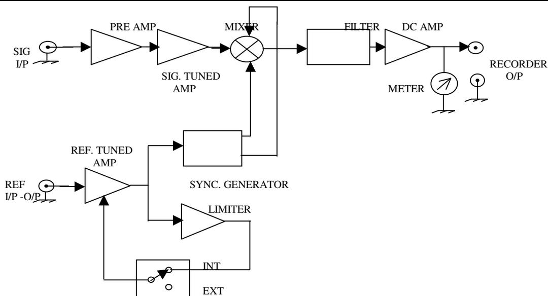
**Figure 2.6** Block diagram of the Lock-in amplifier.
