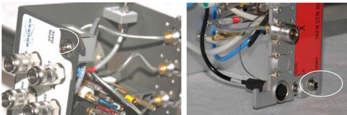
Figure 3.14. Spin Rate Monitor Cable Connector for 2 Different Types of SB Probes
