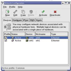
• On the tab pane **Devices** click on *eth0* and click **Edit**. Note that it is necessary to use *eth0* for your internet connection, because *eth1* is required for your spectrometer network connection.
