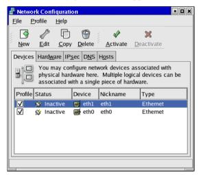
• On the tab pane **Devices** click on *eth0* and click **Edit**. Note that it is necessary to use *eth0* for your internet connection, because *eth1* is required for your spectrometer network connection.
