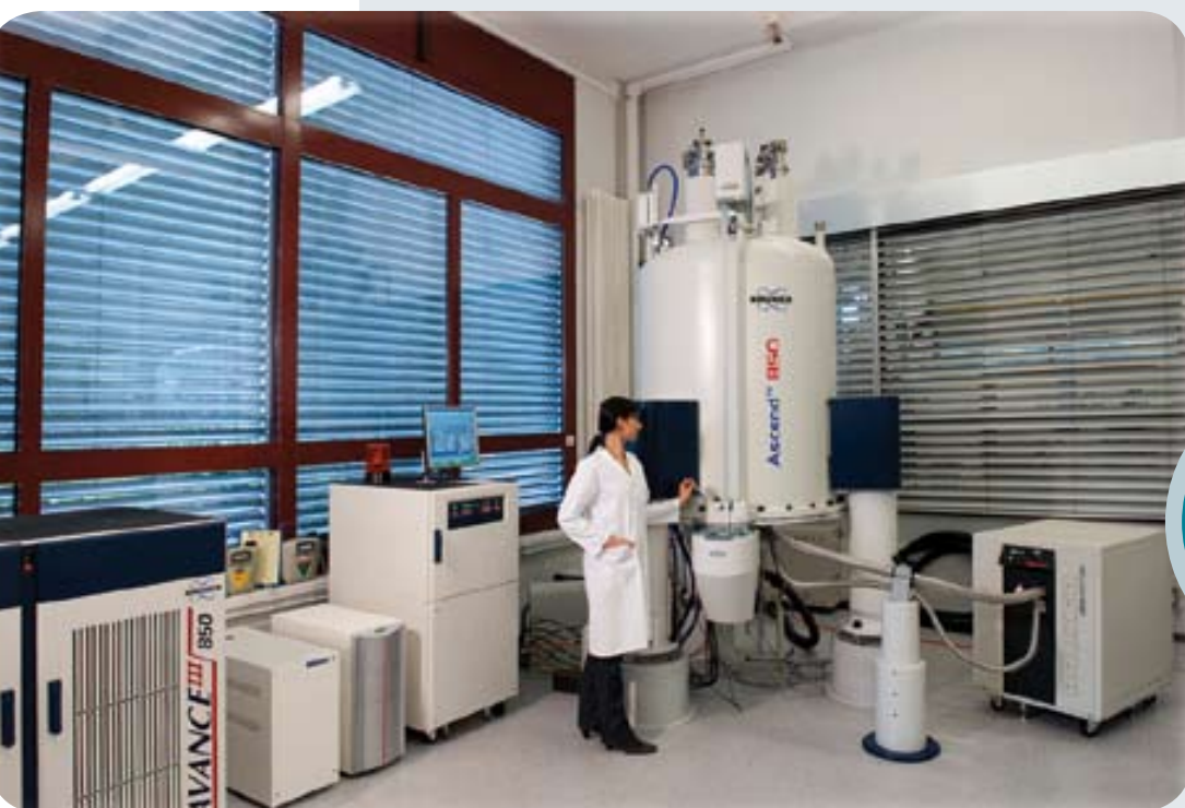
Ultra-High Field Avance III 850 MHz NMR system
